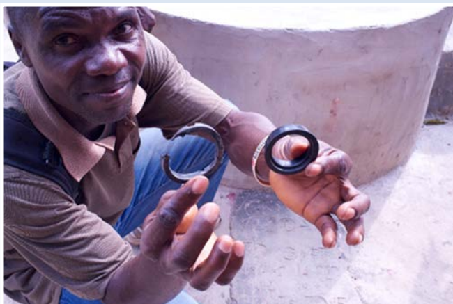
Fred Kermah with a deteriorated O-ring (left) from one of the local wells
